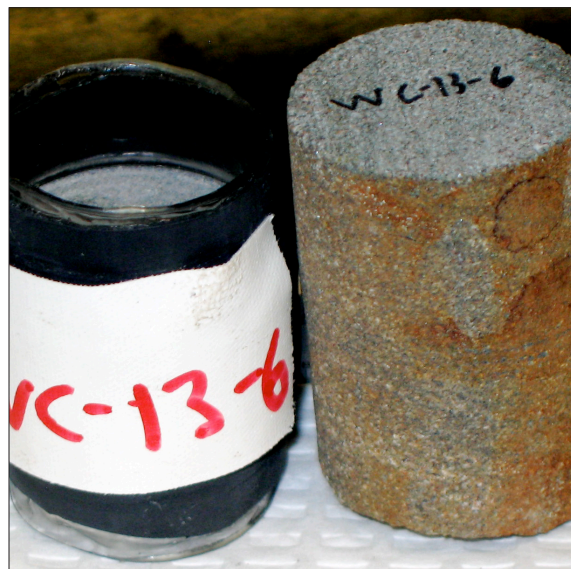
Figure A1.35 Geologic map of northern Wisconsin showing the location of sample WC-13-06 and photograph of core section and thin section used in analysis. Cores are 1 inch in diameter.
