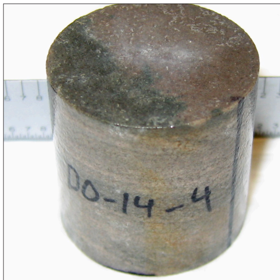
Figure A1.22 Geologic map of northern Wisconsin showing the location of sample DO-14-04 and photograph of core section used in analysis. Cores are 1 inch in diameter.
